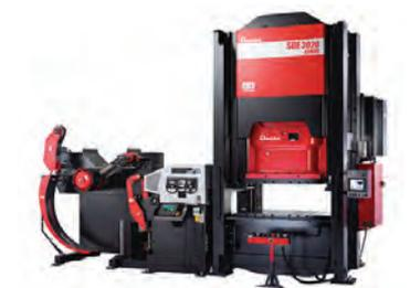
Advanced direct drive servo press offering a highly rigid solid-column frame and full length center-gib with a wide slide. Ranges in size from 150 - 300 mt.
