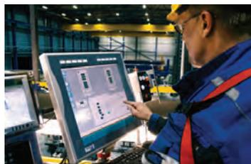
PEMA WeldControl streamlines the communication between operator and machinery during welding operations. Production data monitoring, diagnostics, tracking, and robot programming can be performed by one operator on a one-panel control system.
