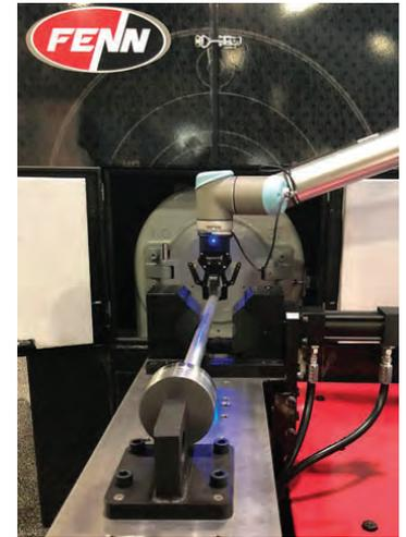
Fully integrated turn-key rotary swaging solution complete with robotics, a sound enclosure, a hydraulic feeder table, and a FENN 3F swager. Benefits include improved equipment safety, reduced set up time and reduced operating costs.
