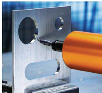
The pneumatically-actuated Compliant Deburring Blade excels in light and medium deburring, chamfering, and scraping operations. Both axial and radial compliance reduces robot programming time and enables consistent contact forces throughout the process.
