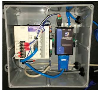
Connect fabricating equipment with the Status Relay Control (SRC) - any machine, brand and age of equipment.
