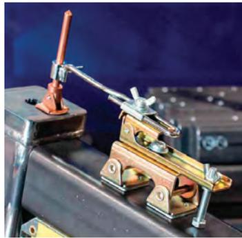
The Deluxe Magnetic Grasshopper locates and holds steel stock in the vertical position for tack welding. The spring-loaded Grasshopper arm delivers positive, self-adjusting holding pressure with a copper spindle for grounding contact.
