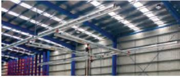
A modular, lightweight system that adapts to any environment. No need to upgrade existing structures to achieve handling loads up to 1 ton and the extendable systems can grow with business.
