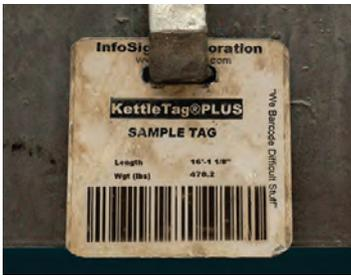
Galvanizing tags with text and bar codes that survive the entire galvanizing process.
