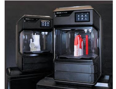
The MakerBot METHOD X manufacturing workstation prints with real ABS, a 100°C build chamber, and SR-30 supports to deliver dimensional accuracy, precision, and reliability.
