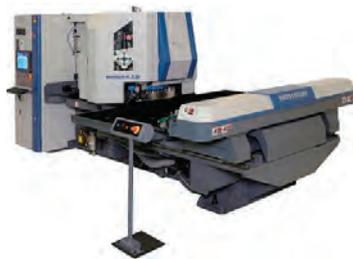
This 22-ton, punch press, uses a servo-electric drive system for simple and reliable processing. A large turret provides flexibility and a small table for limited space. Paired with the RL1212 load/unload system, the punch can work for hours unattended.
