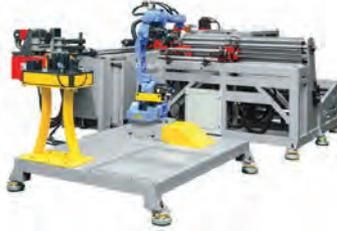
Demonstrates automatic loading, robot unloading, and complex shape inspection and will feature programmable Servo Pressure Die Assist, which will reduce set-up time and operator skill level, as well as control wall thinning and deformation of bend.
