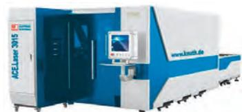
The KNUTH ACE Laser 3015 2.0 has a 5' x 10' cutting table, 2 kW IPG fiber laser source, Precitec cutting head, CypCut CNC control software with nesting function and automatic shuttle table.
