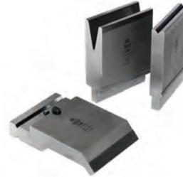
Expanded Wila Trumpf Style press brake tooling with over 30 punch and die profiles. Additions include punches with acute, sash, gooseneck and blade profiles. 55mm height dies have a wide range of V-openings and angles at 30°, 80° and 86°.
