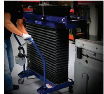
With its easy-glide rollers and hand-pump hydraulics, the Xtreme Lift is one of the safest and least strenuous options to help operators load tools into a press brake.
