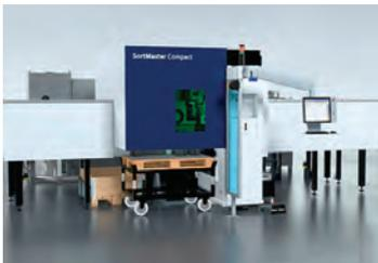
The TruMatic 1000 fiber increases the range of automated production with the SortMaster Compact. The SortMaster Compact removes, sorts and stacks individual parts up to 24" x 16" and up to 33 lbs.
