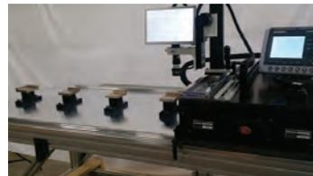
Large format measuring table capable of locating any point in X, Y space for Quality Control checks. Accuracy within +/- .005 inches for non-contact systems. Ranges up to 35x120 inches. Ideal for all part formats up to 4 inches thickness.
