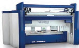
The Advanced Handling System features the dynamic combination of automatic tool change, up and down bending, and automated part manipulation fully automating the entire bending process.
