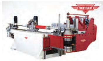
The Herber 2400S is capable of bending up to and including 4" Stainless Steel tubes and was designed for the rigors of high production while offering a
