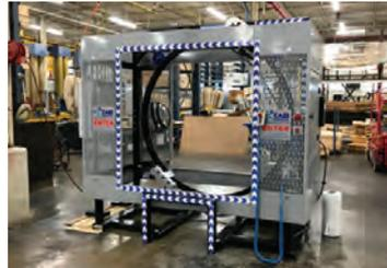
The Smart Control package uses a position encoding system to automatically set the dispensing unit at its home location in the wrapping ring, apply the plastic film, then cut it, holding onto the stretch-wrap for the next pallet load.
