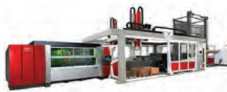
Fully integrated system provides seamless communication between the laser and the sorting mechanism.
