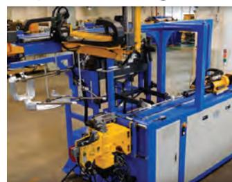
CNC tube bending work cell that demonstrates automatic loading and programmable unloading without the use of a robot. Utilizes X, Y, and Z pick and place
