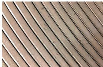
Athader's double eccentric slitter head produces a clean strip edge with minimal penetration, enhancing the edge quality of cut strips and reducing wear on the slitter knives and motor.
