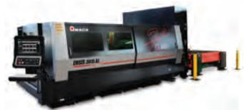
9kW ENSIS fiber laser technology utilizes a collimation system so fabricators can process both thin and thick materials without a cutting lens change or manual setup.
