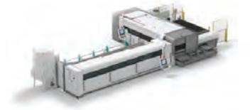
LS5 is one of the markets most complete solutions, designed to evolve with needs. The very compact and configurable layout can be suited to fit available space and processing requirements.
