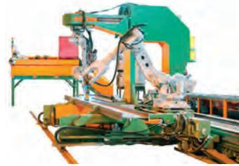
The PeddiAssembler is a robotic steel beam assembly and welding machine which can achieve up to 15,000 tons of completed members per year.
