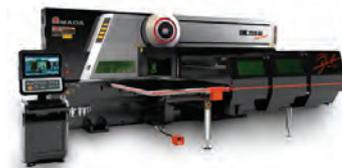
Amada's most popular combination machine pairs the multi-purpose turret with the unlimited shape cutting flexibility of a fiber laser. This grants fabricators the flexibility to work with their customers to create better part designs.
