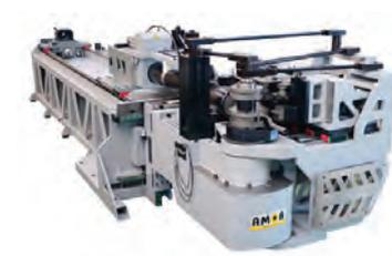
All electric 10-axis multistack boosted CNC bending machine with an extremely large variety of included options.
