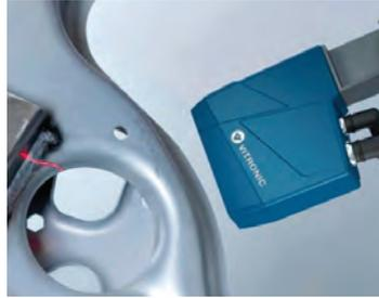
With newly developed sensors, the automated weld seam inspection is even faster and more compact and has been optimized for MIG/MAG and for laser seams.
