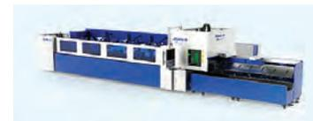
Expert-class ultra-high speed intelligent machine tool with an automatic loading and unloading system that can easily handle a variety of tube shapes and fully covered with protection.
