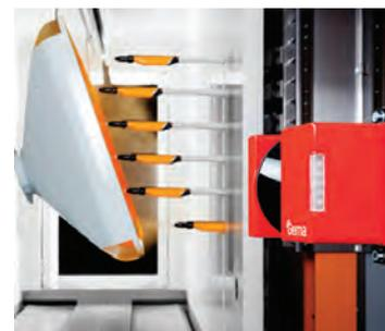
The Dynamic Contour Detection laser scanner offers a higher level of automation for powder coating. The innovative design detects object geometries, aligning each gun to the correct position to coat the most complex components.
