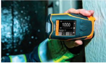
A handheld dry film thickness gauge for coating thickness measurement on steel and non-ferrous metals. Measuring ranges: 0-2500 µm on FE and 0-2000 µm on NF (DFT).
