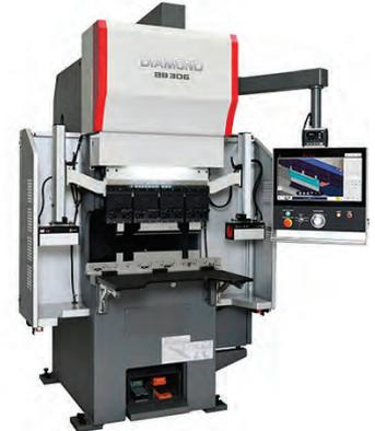
Diamond BB Series Electric Press Brake with AC Servo motor and ball screw mechanism for high-speed productivity and repeatability ( $\pm 0.001\text{mm}$ ).
