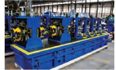
Complete Tube Mill Line equipped with (all new): Kent Corporation Entry Equipment, 300 KW Solid State High Frequency Welder, SFM Forming and Sizing Mills, UCG High-Speed Flying Cold Saw and 3 Motor Drive System.
