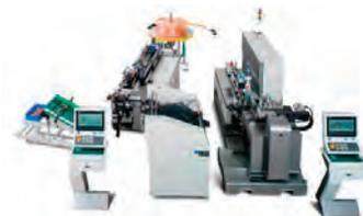
Straightening, end forming, cutting. The 3-RUNNER is a complete tube production process starting from a coil which, straightens, forms (up to six stations), faces, cuts and unloads the finished part. All in one continuous operation.
