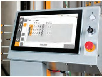
MagicControl® 4.0 provides full control for all automation aspects such as guns, reciprocators and booths for powder coating systems. This allows complete operation of the coating line and consistent process reliability.
