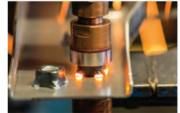
Capacitive Discharge (CD) power supplies equipped with Multi-Capacitor Source (MCS) system.
