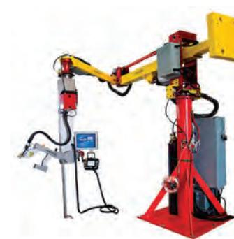
A collaborative welding machine designed specifically for pipe, small pressure vessel, and other types of roll welding. It is capable of welding flanges, tees, elbows, reducers, and more.
