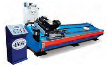
High-Speed Flying Cold Saw equipped with motion controls, length control system, hydraulic clamp system, 325 FPM maximum speed, .160" (4 mm) maximum wall thickness.
