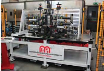
The MTS tube punching and forming units, work plates and machines when combined in work cells can utilize the combination of standard machinery for an almost endless variety of applications such as cutting, single or twinhead bending, punching, forming, flattening, coping, milling and drilling.
