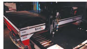
The KANO™ is available in six machine sizes and is configured with a Hypertherm EDGE® Connect CNC, a Hypertherm® high definition plasma system, optional oxy-fuel cutting torch and choice of cutting table style.
