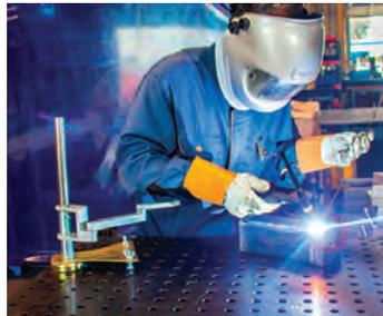
Maximize comfort, productivity and safety in welding with the ReadyRest™ line of Wrist and Arm Rests. The articulated Arm Rest supports the extended arm for greater weld control and complete freedom in positioning.
