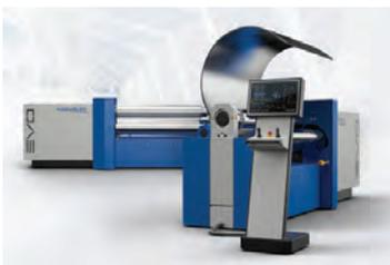
EVO four-roll plate bending machine includes as standard the latest graphically supported CNC Control BENDtronic®, the VSA® variable side rolls swing arm technology and the HAEUSLER Hybrid Drive System HHDS®.
