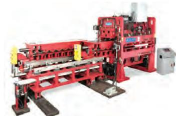
Roll plunge based on gauge and yield, positions machine for desired plastification. Real time roll bending corrects strip defects. Auto side shift cassette change. 4-HI machine allows for 5 or 6-HI with no mods required.
