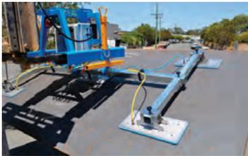
Vacuum lifter to enhance safety when lifting or moving material. Design features, significant modifications and advancements to the vacuum system include an internal self diagnostic vacuum checking and component identification system.
