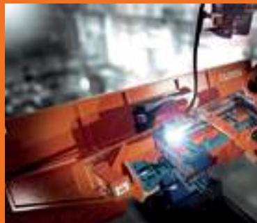
spatter formation at high welding speeds, the MoTion Weld processes are particularly suitable for thin plate applications.
