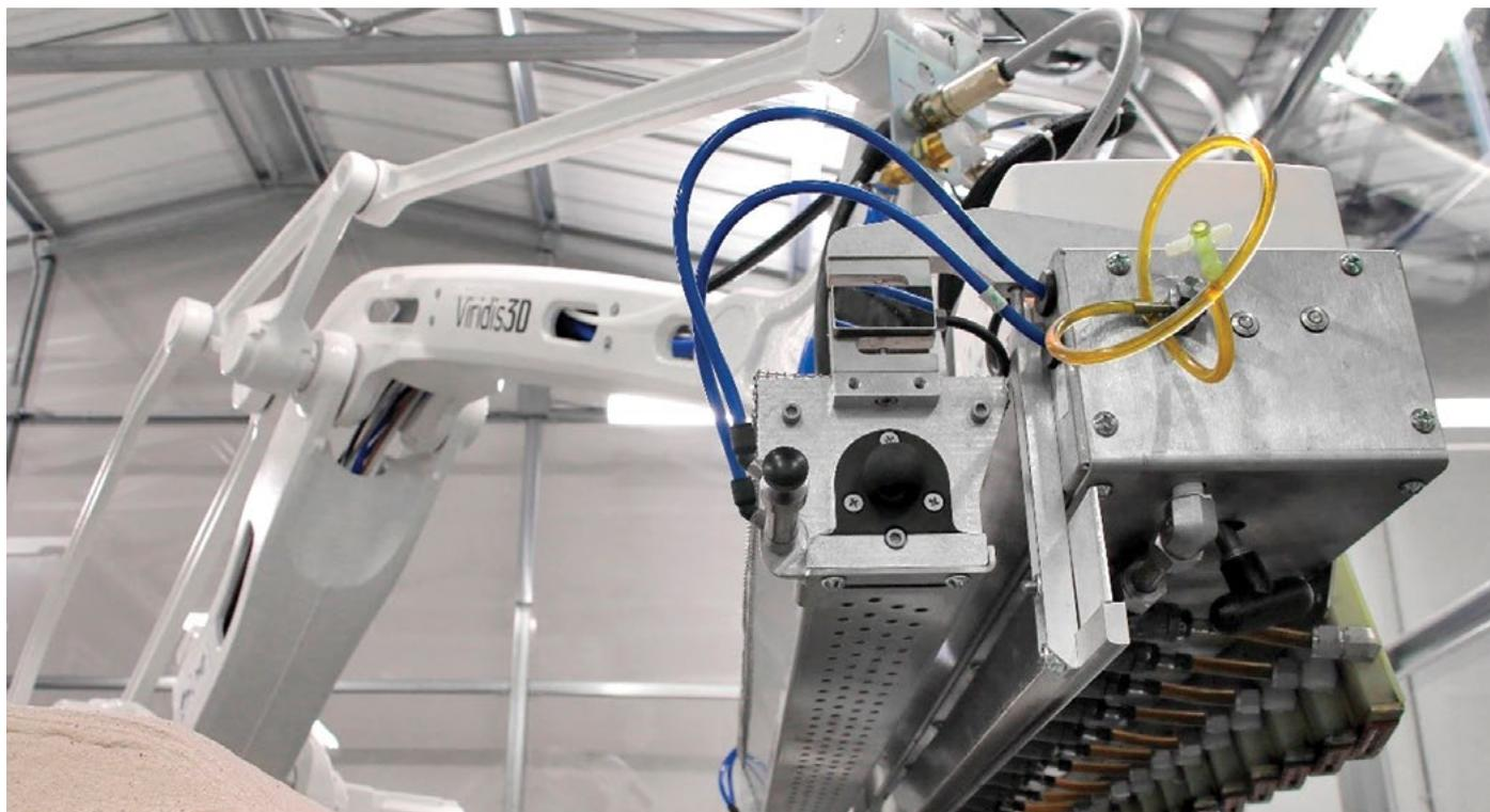
The EnvisionTEC Viridis3D 3D printer has a print head attached to a robot arm. It uses binder jetting technology to print sand molds and cores for the foundry industry. Courtesy of EnvisionTEC
