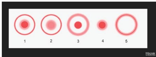
Figure 2: Example 1 shows 50% power in the center core and remainder of the laser power is on the ring core. Example 2 is much more power on the outer ring core and only a little bit of power on the center core. You can see how this power distribution changes.
