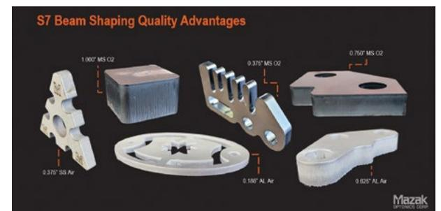
Figure 3: From left to right: 0.375” stainless steel with high performance air, 1.000” mild steel with oxygen, 0.188” aluminum with high performance air, 0.375” mild steel with oxygen, 0.750” mild steel with oxygen, and 0.625” aluminum with high performance air.
