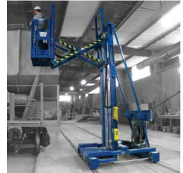
Freestanding 3-axis lift systems allow operators to work on large products by moving the platform lengthwise, elevating, and extending out. Track guided, these lifts can be designed to fit specific applications and are suitable for hazardous locations.
