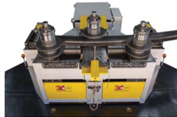
J&S Machine introduces the CLOMEA roll benders with a new line of control options. The bender has 3 driven rolls with 5 adjusted shaft distances for bending up to 5-1/2" tube. A bender can use 6 control models to upgrade as needs and requirements grow.
