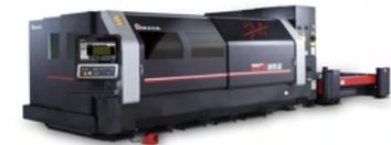
VENTIS utilizes Locus Beam Control (LBC) technology to create infinite locus patterns - ensuring optimum beam shape for each cutting application. This results in the highest quality cuts on stainless steel and aluminum with virtually no dross.
