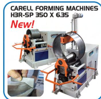
H3R-SP 350 x 6.35 Forming Machines are designed to form a pattern in pre-rolled and welded seam tubes to a specific pattern in 3 tube widths. They incorporate a top roll & pinch roll fitted with hardened profiled rings that form the final part.
