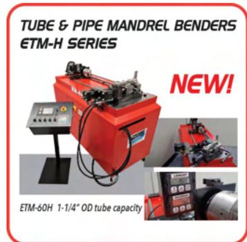
The ETM-H series semi-automatic bending machines perform bending automatically, while the feeding and rotation of the tube is performed manually. Providing a compact, high-performance and economical solution for any shop.
