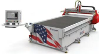
The KANO™ HD 510 Plasma System has a unitized design and heavy-duty steel construction of its larger siblings (up to a 10' x 24' table) with speeds up to 1,500 IPM and a cutting area of 64" x 124".
