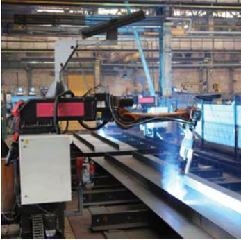
ABAGY is an intelligent system that combines robots, sensors, and computers with proprietary software. With ABAGY, you can use welding robots even for custom projects and one-of-a-kind parts.
