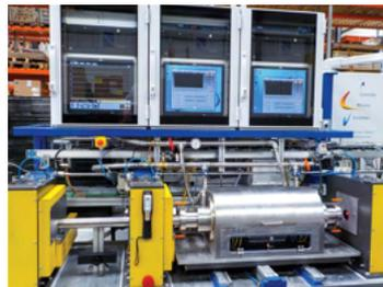
Ultrasonic heads with contactless signal transmission (up to 8000 rpm). Longitudinal & shear waves for longitudinal, transverse, and highly accurate dimensional measurements. A version with phased array electronics is under development.
