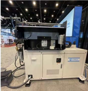
TMS-10WDELU; Comco USA's CNC bender TMS-10 Series with Loader and Unloader.
