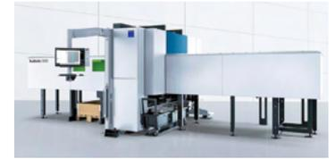
The TruMatic 3000 fiber is the first combined punch-laser machine from TRUMPF featuring a Touchpoint interface, for even easier tool management. The productive machine pairs a "flying" delta-drive punch head with all-tool rotation and a 3kW TruDisk laser.
