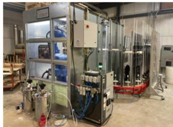
Compact robotic paint systems are for companies looking to automate their paint process with simple and modular automation solutions. Add a robot with simple paint system to existing manual booth or add compact floor conveyor system to increase throughput.
