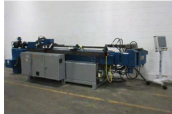
AM Industrial Group can refurbish your Eaton Leonard CNC Tube Bender to create the AMVB300. Refurbished units can include rebuilt valves, rebuilt/replaced hydraulic pumps, new hydraulic hoses, rebuilt cylinders and more.
