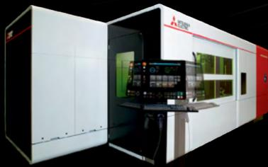
The “brains” behind the **GX-F ADVANCED** Series is the proprietary Mitsubishi Electric artificial neural network technology *Maisart*, which imitates neurons in the human brain. It uses audio and light sensors to monitor the cutting process in real time, automatically adjusting parameters to optimize cutting performance.
