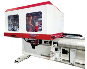
T-DRILL Fully Automatic Collaring Machine SEC-115 with automatic tool changer for five different collaring tools
