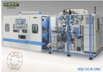
Plant for the production of type BS and K spools for welding wire with or without internal reduction, at a maximum speed of 400 spools/hour.
