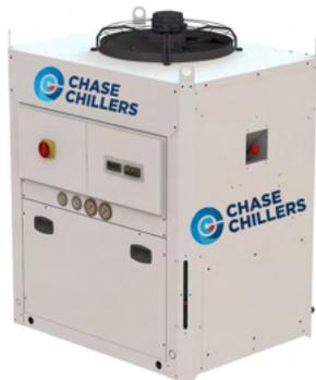
Catered to the laser industry, the QBL017-R expands the QBL Series. Providing just under 6 tons of cooling, the unit has dual cooling circuits with pump flows of 12.9 & 0.5 gpm. Each fully independent circuit can be set to different temperatures.
