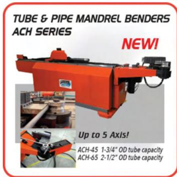
Carell introduces its New Line of “ACH” CNC Mandrel Benders including 2 Models, ACH45 1-3/4” & ACH65 2-1/2” with up to 5 CNC controlled Axis, servomotor controlled bend angle, DBB, POB, 2 stack for-
