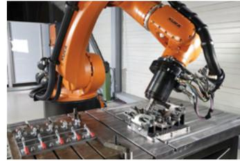
Complex Challenges Solved with Robotic Friction Stir Welding. Friction stir welding is the optimal joining process for non-ferrous metals with a low melting temperature and for mixed-metal combinations.
