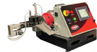
Ideal for solid rod applications up to 0.0625" & up to .25" for tubing. This system includes an automatic feed table and collection bins, and allows for production volume up to 300 pcs/hr. Also minimizes operator involvement, and reduces downstream costs.
