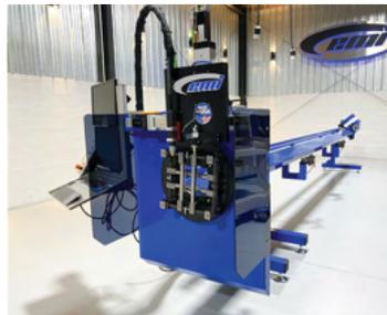
The EL-SQRD is a CNC Plasma Cutting Machine that processes round, square, rectangle, angle, channel, and flat stock. In one smooth, accurate process, you can miter cut, profile, cope, and burn holes and slots in multiple material profiles.
