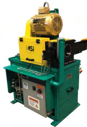
The Model C6H ChamferMate® is a hydraulic-powered pipe beveling machine with up to 6-5/8” OD capacity. With 15 horsepower, the C6H has the ability to machine weld bevels and other forms on the end of heavy wall pipe and tubing within its range.
