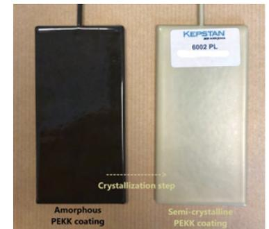
KEPSTAN® PEKK 6002 PL is a high performance thermoplastic powder coating, based on Poly-EtherKetoneKetone (PEKK). KEPSTAN® PEKK is a member of the PAEK family with a lower melting point and Tg close to 160°C, which allows lower processing temperatures.
