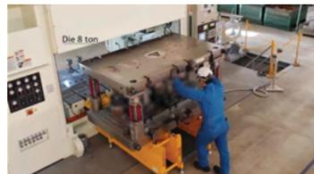
Using a pre-roller stand to load the die with a forklift is easier and has fewer pinch points than loading the die directly into the press. With a pre roller, one person can move an 8 ton die.
