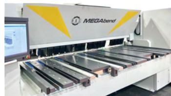
RAS MEGAbend metal folding system offers the precision of updown bending on thick and thin materials. Large-size parts, labor-intensive for press brakes, are ideal for the MEGAbend.
