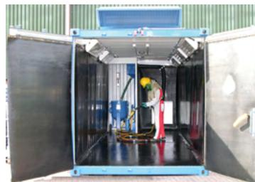
Airblast AFC containerized blast rooms are made from converted shipping containers, which provide an economical solution when a weatherproof and/or transportable blast room is required.
