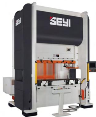
SEYI-America's SD series features the latest servo technology in manufacturing. With full control over every aspect of the stroke, the SD series is excellent for auto parts, consumable electronics, and household appliances.
