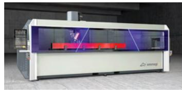
COMET R4 CNC machining center with 5 controlled axes, for machining bars or workpieces made of aluminum, PVC, light alloys in general or steel up to 4 meters long.
