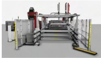
The new ASTES4 SKYWAY is a compact all in one sorting system design to keep up with an ever-changing part demand. With four fully integrated auto-tool-change heads, a wide variety of parts sizes and shapes can be sorted, without any setup time.
