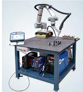
The Lancer COBOT is intended to work side by side with your fabrication's direct human workers within a shared workspace.
