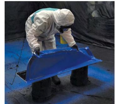
XP-496 is Ultimate Lining's new innovative peelable coating product. It is used to protect products from damage during the shipping and installation of the product. The XP-496's protective coating is easily peeled off once the installation is complete.
