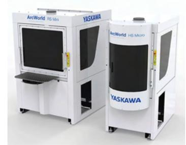
The ArcWorld RS and ArcWorld HS deliver compact and cost-effective options for integrating robotics into current weld processes. Each solution is designed for optimizing small- to medium-size part production for medium volume fabrication.
