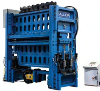
Allor 84" Slitting Line Leveler. Roll plunge based on gauge and yield, positions machine for desired plastification. Real-Time roll bending corrects strip defects.
