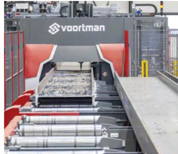
The Voortman V631 adds increased milling capabilities to its proven automated beam drilling machines. Impressive milling capabilities and the ability to simultaneously drill and mark all sides.
