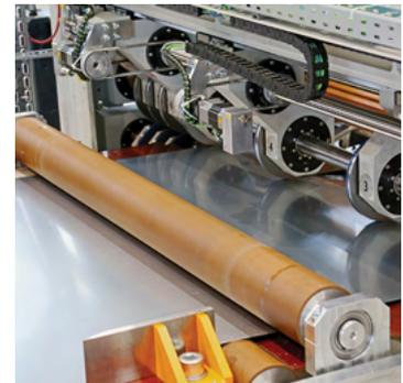
The fully automatic slitting shear for aluminium coils can be easily and flexibly adjusted to new coil widths between 700 and 1,850 mm. As a result, the automatic slitting shear enables short set-up times and quick format changes.
