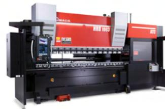
The HRB ATC Series is equipped with AMADA's patented Automatic Tool Changer, making it the ideal solution for variable lot sizes and the seamless introduction of rush jobs.
