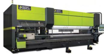
Electronic press brake with automatic tool changer ensures shorter changeover times and time savings when producing small series.
