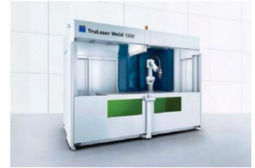
The TruLaser Weld 1000 is an easy-to-use system for fabricators getting started in automated laser welding. The system is well-suited for smaller companies, particularly job shops that weld products like electrical cabinets, sheet metal boxes and covers.
