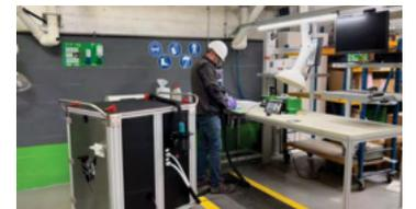
A portable non-drip selective electroplating cart. By using drippless tools, the electroplating chemicals are recycled back into the cart's solution management system - right at the surface of the workpiece without the need for catch trays.
