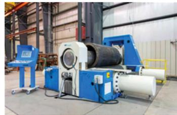
Variable geometry 3 roll bending machine from 1" up to 10" thickness, from 3' up to 20' width.
