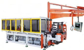
UTE's 3.5" OD all electric bender with shear cutting option. This machine includes multi stacked tooling, shear cutter, and Bendpro G2V3 control. Programmable clamping pressures allow for quick changeover by less skilled operators.
