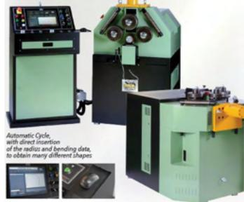
Automatic Cycle, with direct insertion of the radius and bending data, to obtain many different shapes
