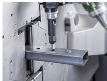
BLM GROUP USA will be launching its LT7 laser tube with a new thread insert unit, which automatically installs thread inserts into laser cut/drilled holes using press fitting.
