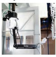
A simple self-learning robotic painting technology mirroring intricate human movements without the need for programming.
