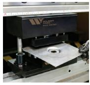
Brake Partner™ lets shops use punch press tooling to make forms in the press brake. This innovative solution can help lower costs and reduce lead times, thanks to the streamlining of equipment and machine flexibility it offers fabricators.
