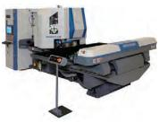
This 22-ton, punch press, uses a servo-electric drive system for simple and reliable processing. A large turret provides flexibility and a small table for limited space. Paired with the RL1212 load/unload system, the punch can work for hours unattended.
