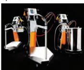
OptiFlex® Pro series brings high performance to manual powder coating. PowerBoost® technology delivers 110,000 volts of power for quick and efficient powder coating.
