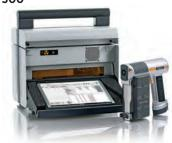
The XAN\*500 X-ray fluorescence instrument can be used as a handheld device, as a fully enclosed desktop unit or integrated directly into production lines. Coating thickness measurements with WinFTM\* software is based on the fundamental parameter analysis.
