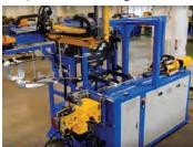
CNC tube bending work cell that demonstrates automatic loading and programmable unloading without the use of a robot. Utilizes X, Y, and Z pick and place unit. This unit is programmed via the bender controller.
