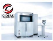
Powder Bed Fusion laser sintering machines.
