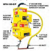
The HFH-100-E/P is a heated 150 pound (or larger) low-mount flux hopper and separator that automatically transfers recovered flux to the welding torch for continuous welding and flux recovery operation. Used with the Mighty-Mac Super Duty Vacuums.
