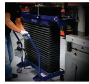
With its easy-glide rollers and hand-pump hydraulics, the Xtreme Lift is one of the safest and least strenuous options to help operators load tools into a press brake.
