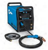
Built for professionals in the light manufacturing or fabrication segments, this smaller, more versatile machine is capable of welding metals up to 1/2-inch thick with an output rating of 230 amps and 25.5 volts at a 60 percent duty cycle.
