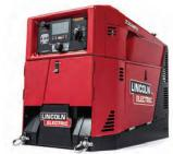
The Ranger® 330MPX™ welder generator is equipped with a 25 horsepower Kohler® engine to supply incredible power for every job. A digital user interface makes set-up easy while offering 10kW of clean AC continuous power. Use CrossLinc® Technology to adjust settings remotely.
