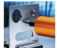
The pneumatically-actuated Compliant Deburring Blade excels in light and medium deburring, chamfering, and scraping operations. Both axial and radial compliance reduces robot programming time and enables consistent contact forces throughout the process.
