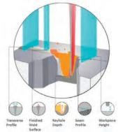
In-line weld monitoring system uses in-line Coherent Imaging to confirm quality of welded parts in real-time. An IR laser beam fired through the same optics as
