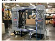
The Smart Control package uses a position encoding system to automatically set the dispensing unit at its home location in the wrapping ring, apply the plastic film, then cut it, holding onto the stretch-wrap for the next pallet load.
