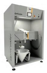
Powder center combining powder feeding, control and electrostatics. This space-saving design provides fast color changes, stable coating results, clean working conditions and trouble-free maintenance.
