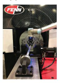
Fully integrated turn-key rotary swaging solution complete with robotics, a sound enclosure, a hydraulic feeder table, and a FENN 3F swager. Benefits include improved equipment safety, reduced set up time and reduced operating costs.
