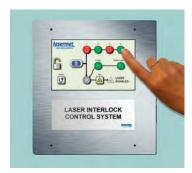
The SLIC is the latest touch screen operated laser interlock control system that connects to the main interlock controller (ICS-7-SP) via an RS232 link. The interlock will only enable the laser to fire once all switches and doors are closed.
