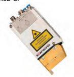
Optical seam tracking sensor using a combination of laser lines and cameras allowing the course of the welding seam to be tracked and corrected in real-time on the Y and Z axis.
