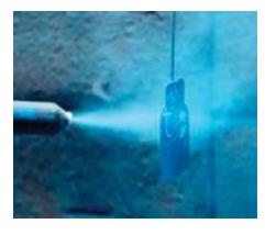
Finishing Pavilion, as directed by their card, to have their part pretreated in preparation for powder coating. Next, they will be able to powder coat the part themselves and before observing the final step in the process, curing. Once the part is cooled, they can take the souvenir part home with them.
