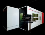
The "brains" behind the **GX-F ADVANCED** Series is the proprietary **Mitsubishi Electric** artificial neural network technology **Maisart**, which imitates neurons in the human brain. It uses audio and light sensors to monitor the cutting process in real time, automatically adjusting parameters to optimize cutting performance.
