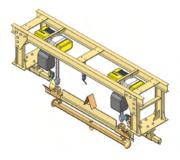
NikoTrack's Drop-Lift devices allow for an inline lifting station for loading/unloading parts onto an overhead conveyor.
