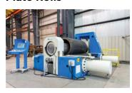
Variable geometry 3 roll bending machine from 1" up to 10" thickness, from 3' up to 20' width.
