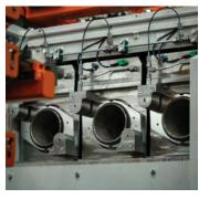
Monitor and optimize vour tube drawing process with the Optimizer4D by QASS. Our device detects premature signs of chatter and reduces the drawing speed proactively before chatter becomes a problem. No more manual speed reductions necessary.
