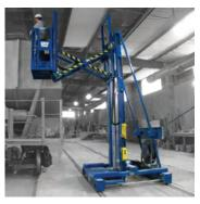
Freestanding 3-axis lift systems allow operators to work on large products by moving the platform lengthwise, elevating, and extending out. Track guided, these lifts can be designed to fit specific applications and are suitable for hazardous locations.
