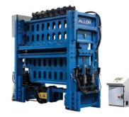
Allor 84" Slitting Line Leveler. Roll plunge based on gauge and vield, positions machine for desired plastification. Real-Time roll bending corrects strip defects.
