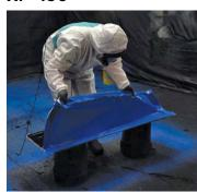
XP-496 is Ultimate Lining's new innovative peelable coating product. It is used to protect products from damage during the shipping and installation of the product. The XP-496's protective coating is easily peeled off once the installation is complete.
