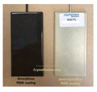
KEPSTAN® PEKK 6002 PL is a high performance thermoplastic powder coating, based on Poly-EtherKetoneKetone **KEPSTAN®** (PEKK). PEKK is a member of the PAEK family with a lower melting point and Tg close to 160°C, which allows lower processing temperatures.
