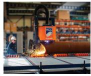
New ProCutter900 RB provides total process pipe-cutting productivity, automating and streamlining on a small footprint. Cuts precision profiles from 2 to 36-inch diameter pipe up to 42 ft. in length. Integrates an automated material handling system.
