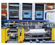
Ultrasonic heads with contactless signal transmission (up to 8000 rpm). Longitudinal & shear waves for longitudinal, transverse, and highly accurate dimensional measurements. A version with phased array electronics is under development.
