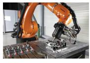
Complex Challenges Solved with Robotic Friction Stir Welding. Friction stir welding is the optimal joining process for non-ferrous metals with a low melting temperature and for mixed-metal combinations.
