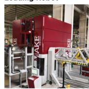
The STAHL slitting tool robot by MAKE is a robot for coil slitting automation that cleans, preps, inspects and preserves your tools, extending their lifespan.
