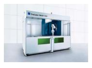
The TruLaser Weld 1000 is an easy-to-use system for fabricators getting started in automated laser welding. The system is well-suited for smaller companies, particularly job shops that weld products like electrical cabinets, sheet metal boxes and covers.
