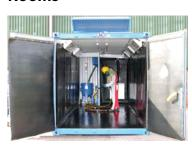
Airblast AFC containerized blast rooms are made from converted shipping containers. which provide an economical solution when a weatherproof and/or transportable blast room is required.
