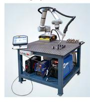
The Lancer COBOT is intended to work side by side with your fabricadirect tion's human workers within a shared workspace.
