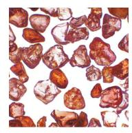
Sourced from top-quality feedstocks, HPR is 100% recycled garnet - processed, screened, and packaged according to stringent standards
