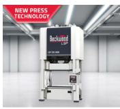
Beckwood LSP™ is a new type of press that uses patent pending linear servo technology to achieve full tonnage throughout the stroke at production-level speeds without hydraulic or mechanical flywheel systems. Models range from 125-500 tons of force.
