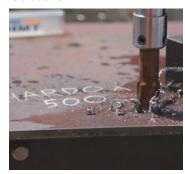
CarbideMax ULTRA cutters are specifically designed for long-life performance in the toughest broaching jobs on the planet, including Hardox steel. Capable of providing a service life in excess of 9x longer than uncoated TCT tools.
