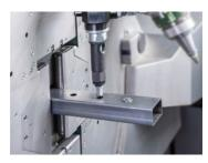
BLM GROUP USA will be launching its LT7 lasertube with a new thread insert unit, which automatically installs thread inserts into laser cut/drilled holes using press fitting.
