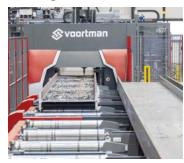
The Voortman V631 adds increased milling capabilities to its proven automated beam drilling machines. **Impressive** milling capabilities and the ability to simultaneously drill and mark all sides.
