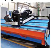
Maximum Outside Diameter: Tube: 3-1/2" (89 mm), Square: 2-1/2" (63.5 mm), Rectangle: 1-1/2" x 3" (38.1 mm x 76.2 mm). Maximum Wall Thickness: .160" (4.06 mm). Thickness: Minimum .030" (.762 mm). Blade Type: HSS-TCT
