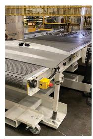
MPI Part Out Conveyors offer a reliable solution to remove stamping press parts. A flexible design adjusts for many die setups - always tracking accurately. A sturdy plastic chain belt is more durable than traditional belt materials saving time and money.
