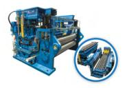
Manufacturing, Allor Inc. introduces our new COMPACT STRAIGHT-ENER. Efficiently feeds the pickle line while utilizing small diameter work rolls for SHAPE CORRECTION and SCALE BREAKING.
