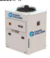
Catered to the laser industry, the QBL017-R expands the QBL Series. Providing just under 6 tons of cooling, the unit has dual cooling circuits with pump flows of 12.9 & 0.5 gpm. Each fully independent circuit can be set to different temperatures.
