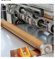
The fully automatic slitting shear for aluminium coils can be easily and flexibly adjusted to new coil widths between 700 and 1.850 mm. As a result, the automatic slitting shear enables short set-up times and quick format changes.
