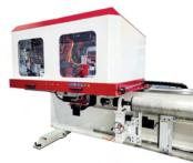
T-DRILL Fully Automatic Collaring Machine SEC-115 with automatic tool changer for five different collaring tools
