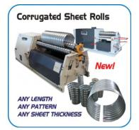
Carell New Series Plate Rolls for corrugated sheet materials now are available to handle all corrugation patterns, lengths, and thickness in any material type. Standard and CNC Controls are available for all models.
