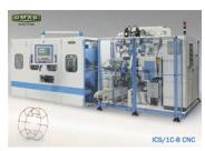
Plant for the production of type BS and K spools for welding wire with or withour internal reduction, at a maximum speed of 400 spools/ hour.
