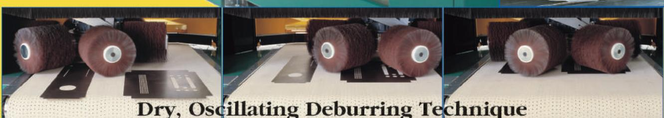
Dry, Oscillating Deburring Technique
