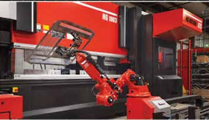
The HG 1003 ARs is designed to handle sheets up to 39" x 31" and the system's robot can support loads up to 44 lbs.
