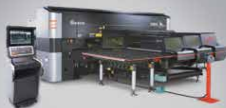
LC 2515 C1 AJ Punch/Fiber Laser Combination
